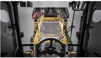
The 432F2 is fitted with Pilot controls providing low effort operation, with the ability to switch between ISO (Excavator) or SAE (Backhoe) control patterns with the press of a button. Providing easy and safe operation for operators of any experience or ability.
